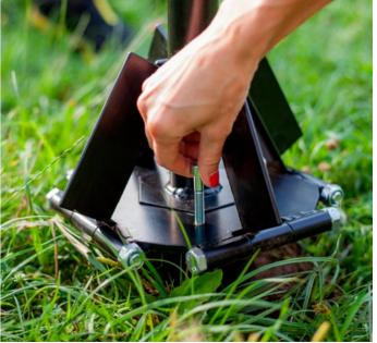
Fold out all four arms of the upper panel and remove all small the small screws.
